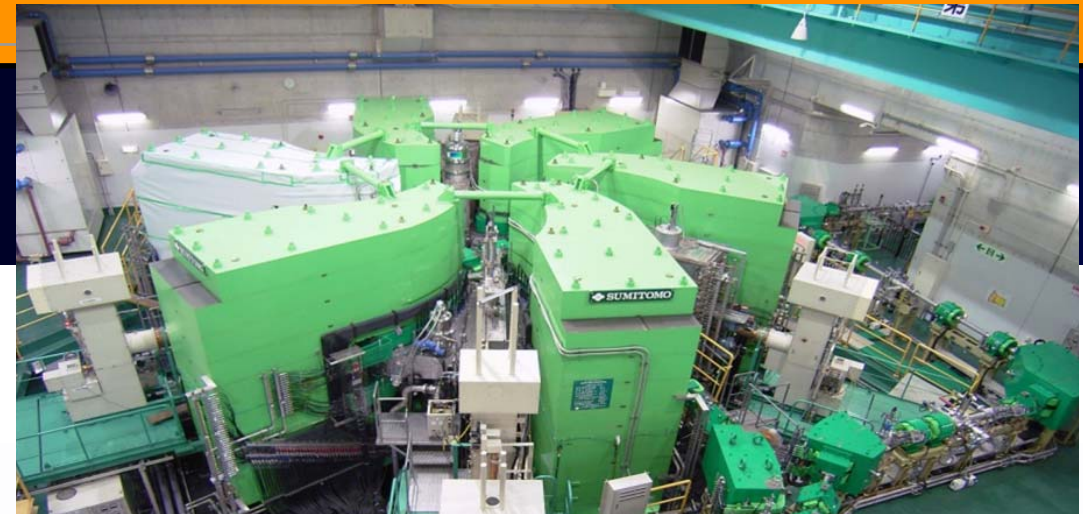
Cyclotron, Osaka University, 1\mu\text{A} , 400 MeV (400W)
